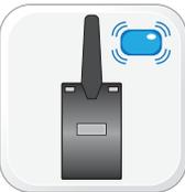
The antenna's leds will flash BLUE once [1x] for each successful pairing.
